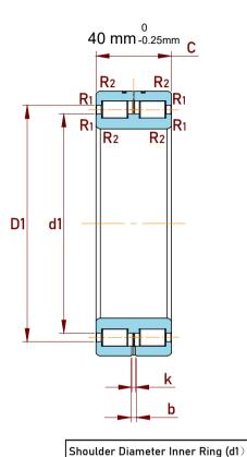
Raceway Diameter Outer Ring (D1)
