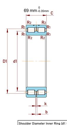
Raceway Diameter Outer Ring (D1)
