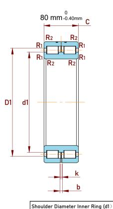
Raceway Diameter Outer Ring (D1)
