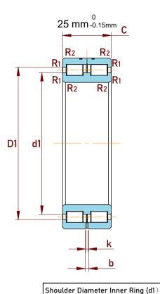
Raceway Diameter Outer Ring (D1)
