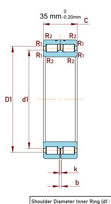
Raceway Diameter Outer Ring (D1)
