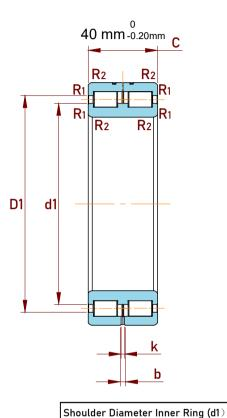
Raceway Diameter Outer Ring (D1)
