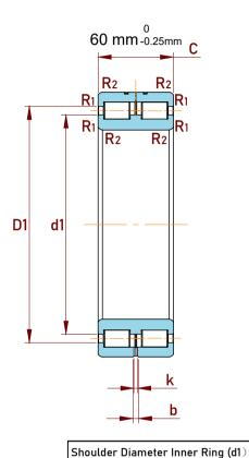
Raceway Diameter Outer Ring (D1)
