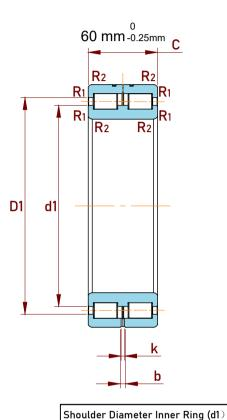
Raceway Diameter Outer Ring (D1)
