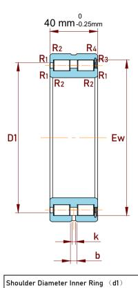
Raceway Diameter Outer Ring (D1)
