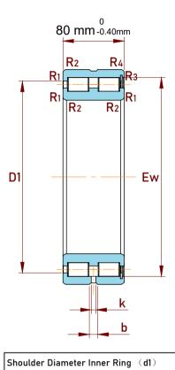
Raceway Diameter Outer Ring (D1)
