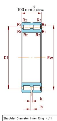
Raceway Diameter Outer Ring (D1)
