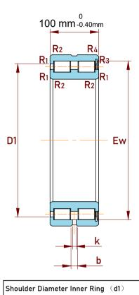
Raceway Diameter Outer Ring (D1)
