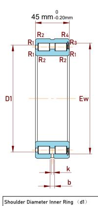
Raceway Diameter Outer Ring (D1)
