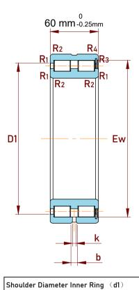
Raceway Diameter Outer Ring (D1)
