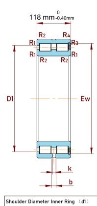
Raceway Diameter Outer Ring (D1)
