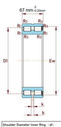
Raceway Diameter Outer Ring (D1)
