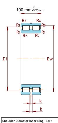
Raceway Diameter Outer Ring (D1)
