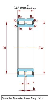
Raceway Diameter Outer Ring (D1)
