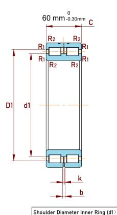
Raceway Diameter Outer Ring (D1)
