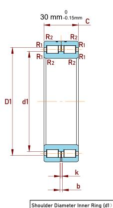
Raceway Diameter Outer Ring (D1)
