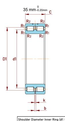
Raceway Diameter Outer Ring (D1)
