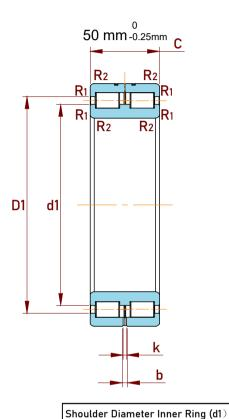
Raceway Diameter Outer Ring (D1)
