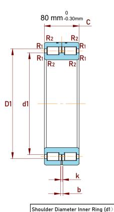
Raceway Diameter Outer Ring (D1)
