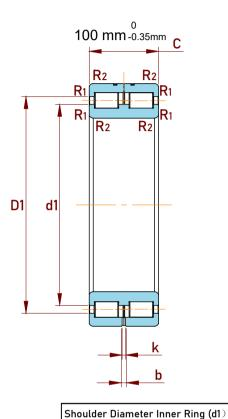
Raceway Diameter Outer Ring (D1)
